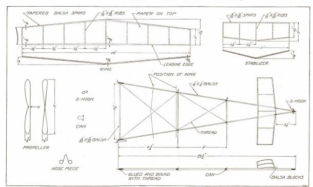
The model is easy to build. It's wise to study both diagram and instructions before starting work, however.
